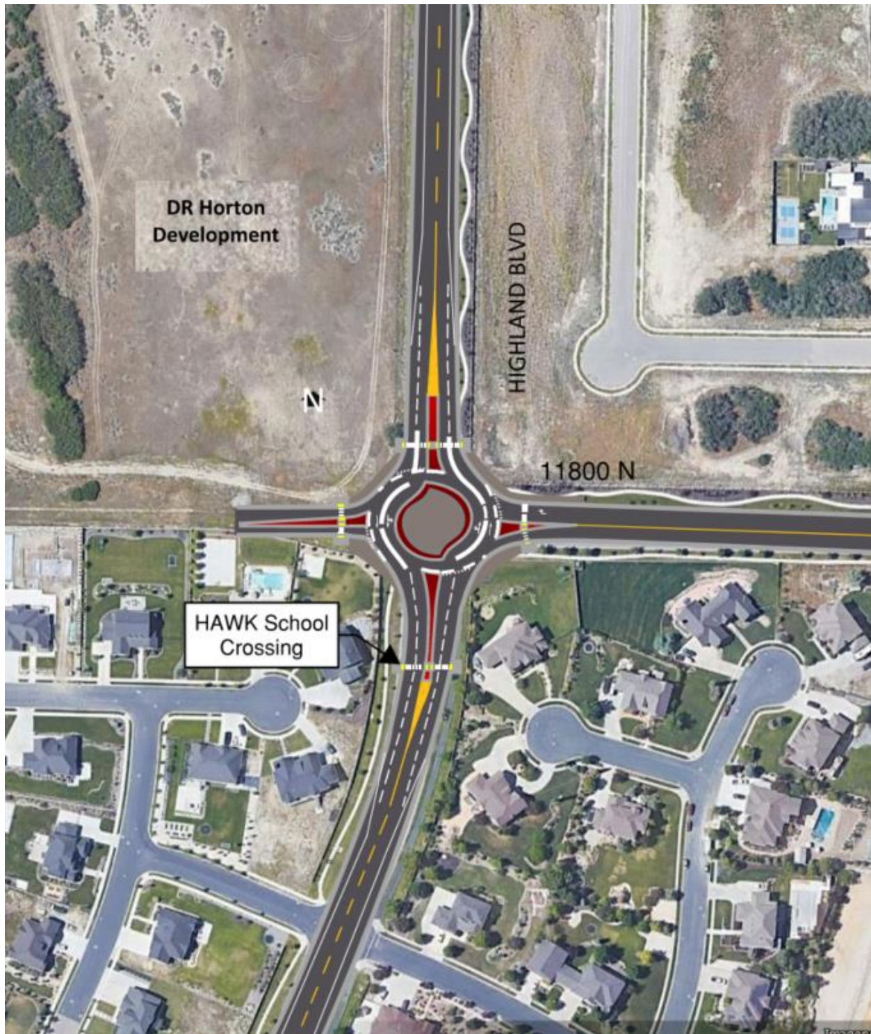
FIGURE 8 - 2X1 MULTILANE ROUNDABOUT - FULL EXTENTS
